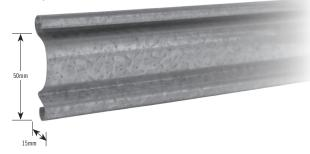
$0.8 \, \text{mm}$ , continuous roll formed, interlocking, coated galvanised steel slats. Nominal effective pitch of 50mm. Zinc coating of not less than  $275 \, \text{g/m}^2$ . The curtain is fitted with moulded nylon clips to the ends of alternate slats by two nylon rivets.
